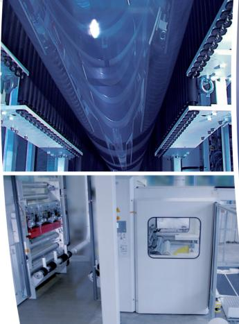
Lines for the production of bi-orientated flat films for high barrier packaging
